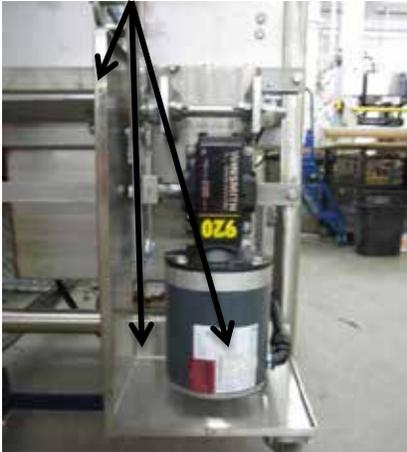
6. Remove greabox from H-Bracket using 9/16" socket (4 nuts)
