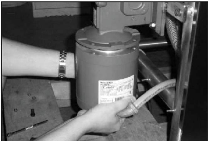
Removing the drive motor.
