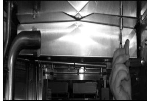
Removing and turning splash shield
