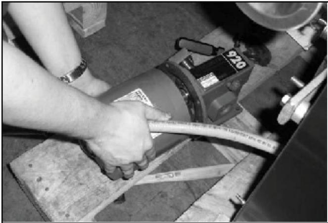
Mounting the motor to the gear reducer.
