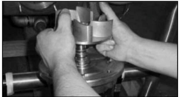
Removing the impeller
